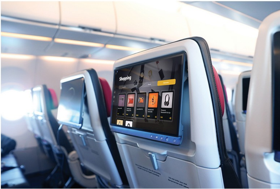
Panasonic's Astrova IFE system features modular architecture for easy hardware and software upgrades. Credit: Panasonic
