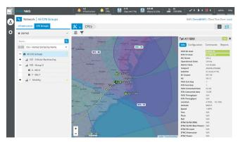
With TotalNMS maps, the geographically-based behavior of mobility services are easily defined and modified. Parameters include VNO service boundaries, areas where transmission is not allowed and the right place to switch between overlapping beams.
