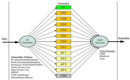
The QoS mechanisms enables the service provider to prioritize specific traffic class defined by flexible rules to ensure performance and to improve end-user experience.
