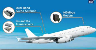
A dual Ka and Ku-band antenna enables service providers the freedom to choose the lowest cost, best performance satellite capacity with almost no practical restrictions. It enables business flexibility to add overlapping Ku-band capacity where Ka-band beams are fully utilized.
