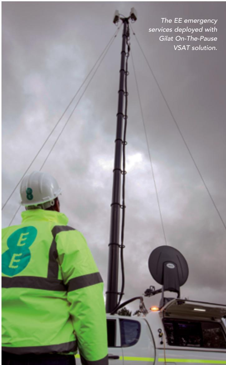
*The EE emergency services deployed with Gilat On-The-Pause VSAT solution.*
