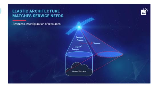
Gilat's elastic architecture also allows dynamic capacity steering of resources between beams to answer real-time changes in terminals throughput demand over specific geographic locations. No longer will it be required to allocate the maximum needed carrier size and compute power ahead of time. The inefficient "design to peak usage" is no longer essential, due to the architecture's elastic nature.
