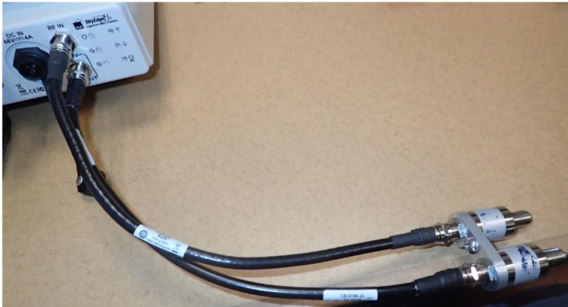
Figure 2: Capricorn MEC Outdoor – Connecting RF Lightning Protection
